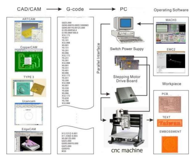
Below diagram shows a typical CNC working flow.
